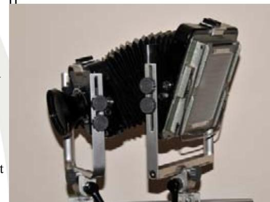
View camera gymnastics! The Arca with shift, swing and tilt movements employed for both the lens board and the back.
