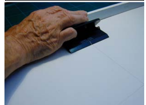
Using the cutter, lining up horizontal edge with blade (white line) on the matt cutter
