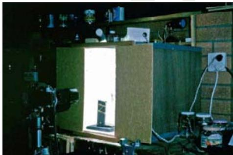
The big job though was to get these backgrounds out of focus in the final picture but well illuminated at the same time. The final size for my studio was 400mm high, 400mm wide and 530mm deep with a sheet of glass for the top. The front doors slid in grooves so that I could open them just enough to poke the lens through and the whole of the inside facing walls plus the base were painted flat white to act as reflectors.
